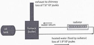
If all the heat from the combustion was used to heat the water, the system would be 100% efficient. However, some heat is lost in the furnace exhaust and some is lost from the pipes delivering the water to the radiators.
